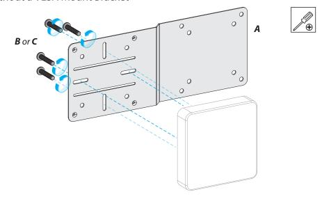
**Note:** Use two Screws on either the vertical or horizontal Short Mounting Slots.
