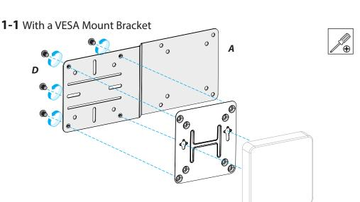
**Note:** Use the specific Screws and VESA Mount Bracket that came with the NUC or Thin Client.
