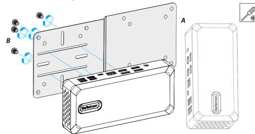
**Note:** Attach the Docking Station in horizontal or vertical orientation according to needs.
